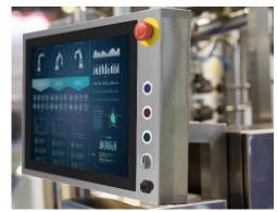
User-defined function push-buttons and rotary switch on front panel
